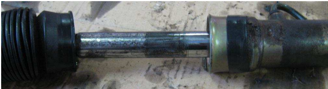
NOT GOOD - Rusty rack
