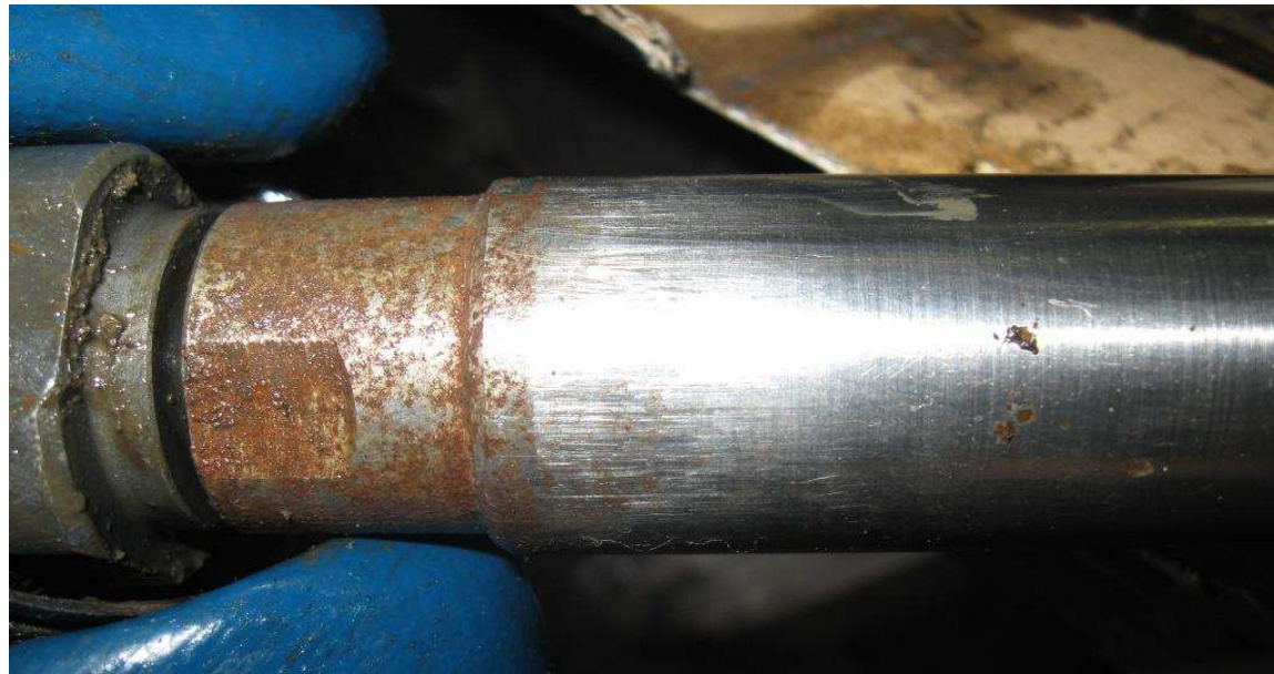
NOT GOOD - Rusty rack
