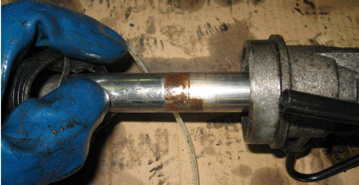
NOT GOOD - Rusty rack
