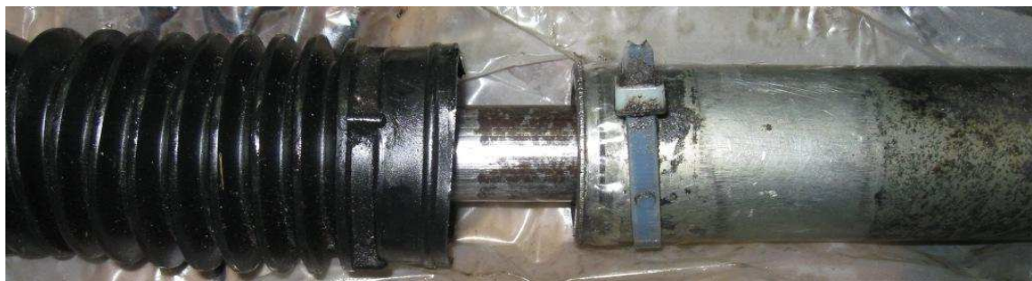
NOT GOOD - Rusty rack
