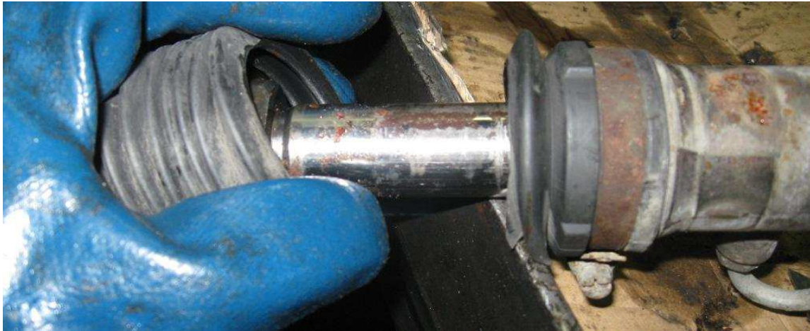
NOT GOOD - Rusty rack
