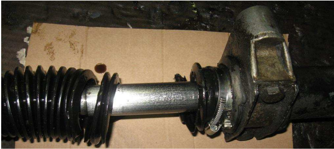
NOT GOOD - Rusty rack
