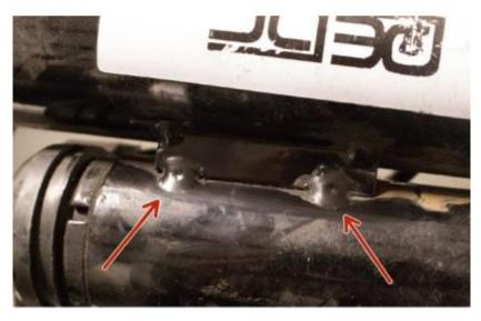
ALS valves (connectors) valves marked as ALS are not OE valves, so the cores they are on are considered as non-OE cores. Only shock absorbers with VOSS valves are considered as OE products.
