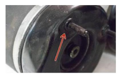
**Spot welded pins** spot welded pins make the core be qualified as a non-OE core).
