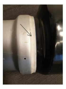
Spot welds spot welds on the valve housing and the shock absorber connectors represent a non-OE part. The only exception where point welds are used is the Mercedes-Benz S-Class W220 (AS-2193 & AS-2194) columns).
